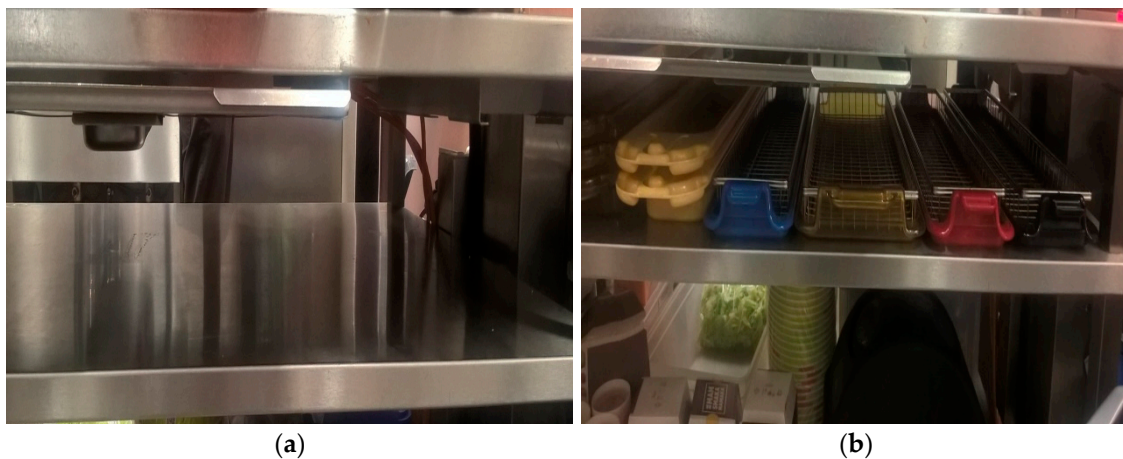
Figure 7. Management of unused space. (a) Free space designated for storage; (b) space managed upon applying the 5S method.
