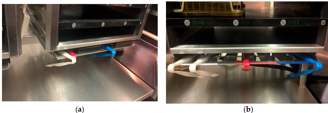
Figure 6. The system of tongs: (a) before applying 5S; (b) after applying 5S.
